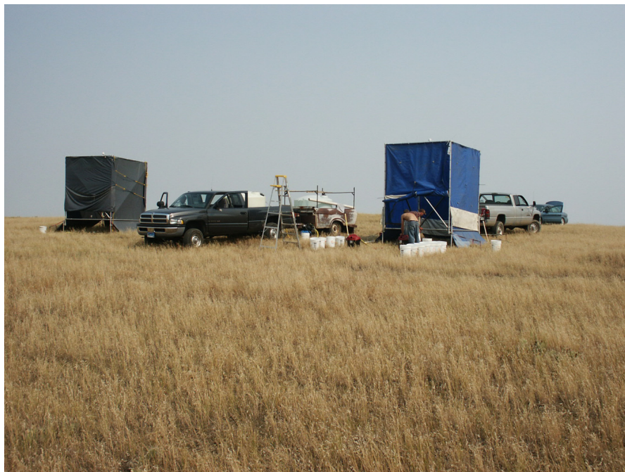
Figure 3-9. Rainfall Simulators for Infiltration and Runoff Study.
